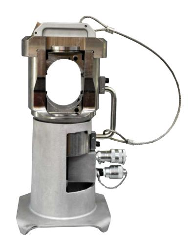
The **EP-60D2** series is a double acting model. Double acting tools will eliminate the possibility of the tool jamming. Double acting means hydraulically advancing the ram to build the proper tonnage, then the hydraulic pressure is reversed to retract the ram. This will ensure the ram to retract without having to pry the jaws apart to release them and it will also retract much faster than single acting spring release tools.
