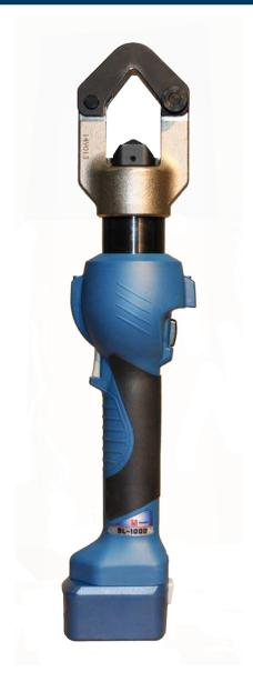
The **SL-1000** is a hand-held, dieless compression tool that is able to crimp connectors up to 1000 MCM copper and 1000 aluminum. The SL-1000 is the first dieless 12 ton streamline compression tool in the industry featuring a latched head design. The dieless indent style crimping head does not require interchangeable crimping dies. The SL-1000 has a release trigger to feather ram for faster crimping cycles and runs off the same Huskie battery that all Huskie Tools use.
