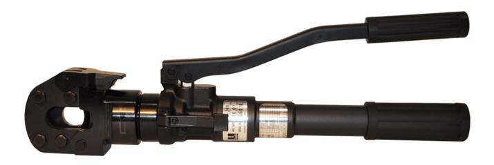
Huskie's **S-Series** tools cut anything from guy wire\* to anchor rod and most overhead and underground cables. The S-series cutters are portable, lightweight, and made to last years under the toughest field conditions. The S-40B and S-85 feature a two stage pumping piston for rapid advance.
