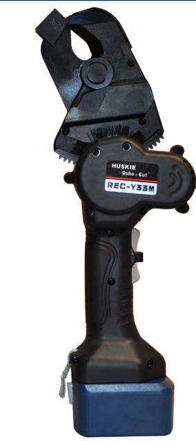
The **REC-Y33M** cable cutter is used to cut up to 636 ACSR and up to 500 MCM\* copper cables. The open jaw makes it easy to insert cables for one handed operation. The jaw, which incorporates a blade retainer, keeps the blade from spreading apart when cutting cable with a steel core.
