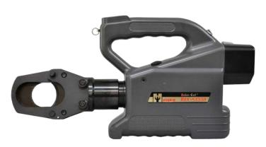
The **REC-S3550** cuts ACSR, guy wire, wire rope, and ground rod. Powerful and portable with a 2" jaw opening. A latch-type jaw swings open to accept material to be cut. The head can be rotated for proper positioning of rod or cable. This is our most versatile cutter patterned after our S-55B hand operated cutter.
