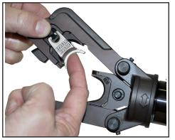
3) Press the trigger to activate the tool and advance the ram so the connector is held between the dies. Once the connector is securely held, place the conductor into the connector.
