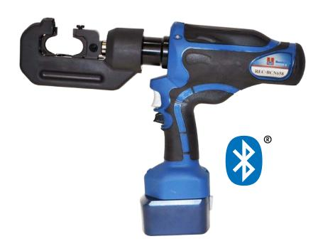
The **REC-BCN658** is an open jaw version of the REC-658U latched type tool. The open jaw can easily fit into tight situations where the closing of a jaw latch would be a problem. The jaw is covered with a rubber boot designed to provide some insulated protection against "brush" contact with energized cables. The tool should not be used as an insulated tool since the dies and die holding pins are always exposed.
