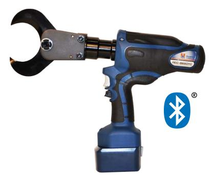
The **REC-B660YC** works well for most underground aluminum cable cutting applications. It was designed to cut copper cables up to 500 MCM\* and aluminum up to 2" maximum outside diameter. The extra wide jaws make cutting the larger diameter underground cables easier. The hydraulic system is designed the same as the REC-658U featuring a rapid advance ram to reduce cycle time.
