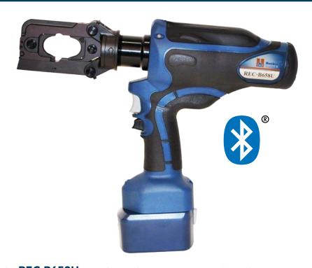
The **REC-B658U** was designed to squeeze commonly used service entrance connectors, including lugs, sleeves, H-Taps and C-Taps. The rapid advance feature allows the operator quicker compression cycles. In addition to the rapid advance feature, it also has incorporated an electronic counter that will allow a service technician to read the number of compression cycles the tool has made. Also, the new tool housing has been reinforced to improve durability during heavy field use.
