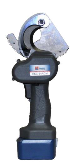
The **REC-54ACM** was designed to cut stranded copper cables and aluminum. The jaws will accept a maximum of 1500 MCM aluminum. The operation of this tool is the same as the REC-54M, but it has sharper blades for cutting only non-ferrous materials. Do not cut steel with this model, or blade damage will occur.
