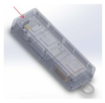
Maintain hands and fingers a minimum distance of 20mm from the device antenna. Antenna shown.
