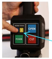
Once the hand held remote is powered on, the blue "paired" LED will illuminate.
