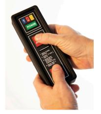
The operator will know the cable is cut when the yellow "blade engaged" LED is off – this indicates the blade has completely gone through its arc and out the other side, leaving no chance the cable has not been cut. If LED is still illuminated, the blade has stopped, and cable is not cut. Cycle time should be approximately 15 to 20 seconds.
