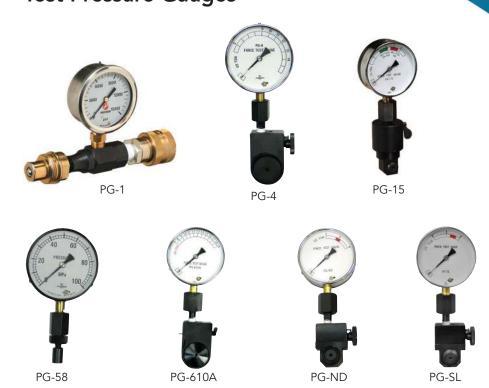
The PG-1, in line pressure gauge has standard 3/8" couplers and a 10,000 psi indicator. It is used to test pump output pressure. Male and female couplers allow you to install it between the tool head and the pump.
