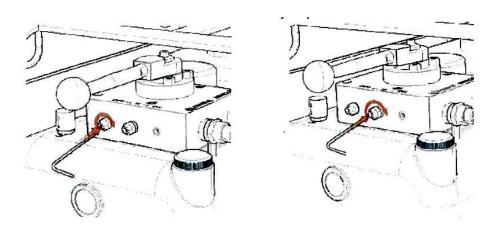
**Note:** An allen wrench is required to adjust the pressure.
