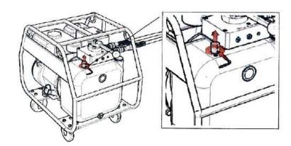
6. Attach proper hoses and make sure they are secure and screwed on tight. When in Single Acting Operation, attach the hose to the port on the pump labeled "Single".
