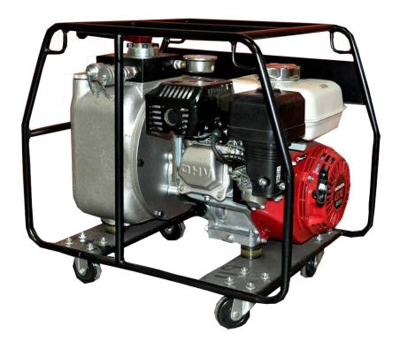
The **HPM-P3** is a self-contained high pressure pump, with manual operation. It is equipped with a 5.5 HP Honda engine. A four-way valve controls the hydraulic fluid direction for the advance and retract modes. One, double-acting tool can be operated or two, single-acting tools at one time. Connection to one port for single acting tools will work since the control valve will dump the fluid when shifted to the neutral position. The pump is very compact and comes with carrying cage.
