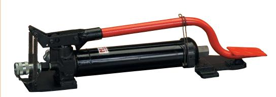
The **FP-700** a portable, tough, hydraulic steel pump that has tow speed pumping pistons for rapid advance and an external adjustable pressure setting from 4.000 to 10,000 psi output. An internal oil bladder allows the tool to be used in any position.
