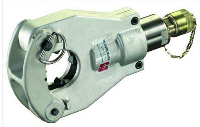
The Huskie **EP-750HA** dieless, Anderson style head has a flip-top opening and a pull-pin locking mechanism to accept larger connectors up to 750 MCM. Output force is 6.2 tons, and 10,000 psi external pumping source is required. The EP-750HA is supplied with a 3/8" male, screw type coupler and a carrying case.
