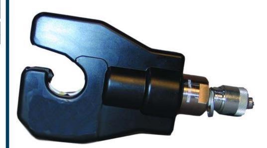
The **EP-630HA** is a dieless remote head that requires an external 10,000 psi pumping source. It is designed to crimp Anderson connectors #10 str - 500 MCM bare Al and #10 sol - 500 MCM bare Cu. The EP-630HA is mostly used by electrical contractors who prefer dieless compression to circumferential compression. This tool is supplied with a 3/8" male, screw type coupler and carrying case.
