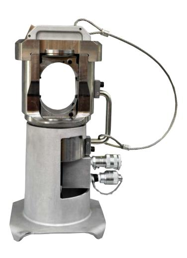
The **EP-60D** series is a double acting model. Double acting tools will eliminate the possibility of the tool jamming. Double acting means hydraulically advancing the ram to build the proper tonnage, then the hydraulic pressure is reversed to retract the ram. This will ensure the ram to retract without having to pry the jaws apart to release them and it will also retract much faster than single acting spring release tools.
