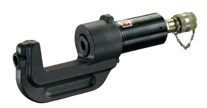
The **EP-510HK** is a Kearney style tool which accepts PH-2, WH-2, and WH-3 style dies. It has 12 tons of output and is used for crimping up to 750 MCM lugs or splices. An external 10,000 psi pumping source is needed to develop 12 tons of compression force. The EP-510HK comes complete with a 3/8" male, screw type coupler and carrying case.
