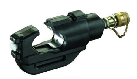
The **EP-510HC** is a remote C-head that requires an external 10,000 psi pumping source. It accepts all "U" type dies used with conventional 12 ton compression tools. The larger jaw opening of 1.65" accepts conductors and mid-span sleeve connections up to 750 MCM. The EP-510HC is supplied with a screw type, 3/8" male coupler, metal carrying case, and die tray. We recommend the use of our non-conductive high pressure hose.
