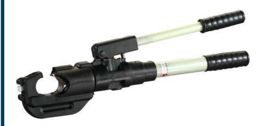
Huskie's **EP-510C** was engineered to accommodate all U-type dies currently used in existing 12 ton tools. It is one of Huskie's most versatile tools since it takes a full range of connectors and lugs to 750 MCM. The jaw opening is 1.65" to accept larger splices up to 750 MCM. The EP-510C output tonnage is adjustable to 14 tons for some specific grounding applications.
