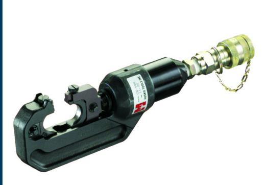
The **CN-58H** remote operated "C" head requires an external pumping source of 10,000 psi. It accepts Kearney "O" type and Burndy "W" type dies. It is a service entrance compression tool and the smallest of our compression tool line. The head is lightweight for easy handling in hot stick applications. The tool is supplied with a 3/8" male screw type coupler and a carrying case.
