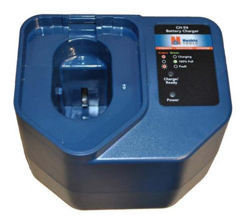
The **CH-94** is a Lithium Ion only charger able to charge the BP-80 and the new BP-82 & BP-84 Huskie Tool Batteries. During its 1 hour charge time, the CH-94 monitors battery temperature and battery voltage for correct charging.
