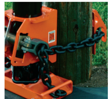
Swivel chain hook assembly is used to pre-tension chain to provide maximum lift per stroke.
